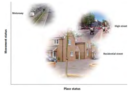
Figure 5.3: Typical road and street types in the place and movement hierarchy (Manual for Streets DfT, 2007)
