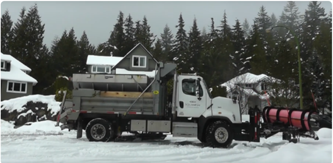
Figure 2.10.1) Image of a M2 tandem axle dump truck typically used for road snow clearing.
