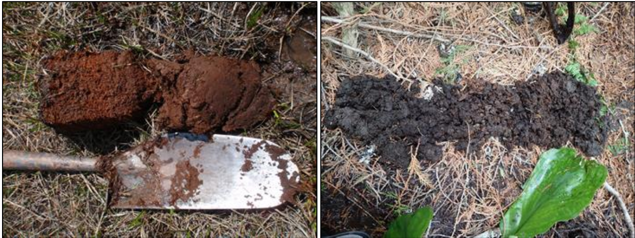
Figure 3. Example fibric peat over mesic peat in a fen (left). Figure 4. Example of a rich mineral soil from a forested swamp (right).
