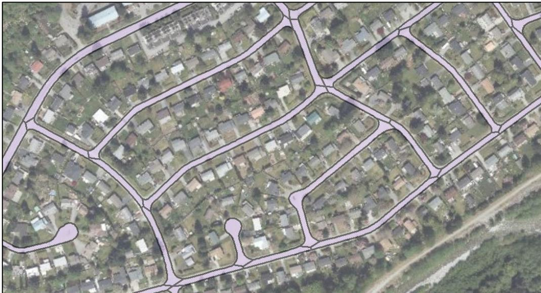
**Figure 5: GIS polygons to collect roadside inventory data**
