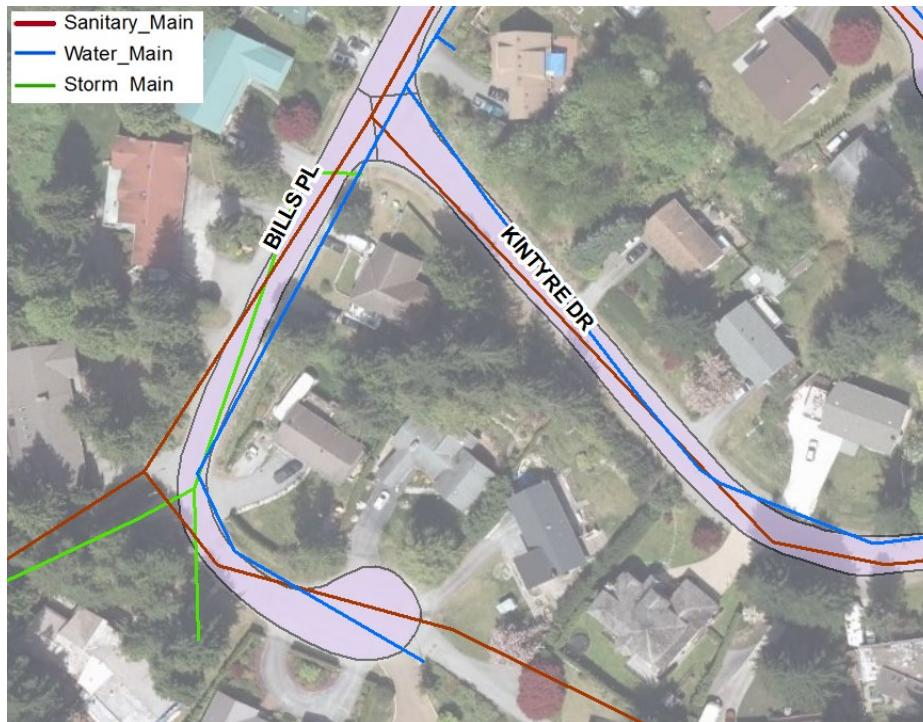
**Figure 6: Underground Utilities Integration in GIS**
