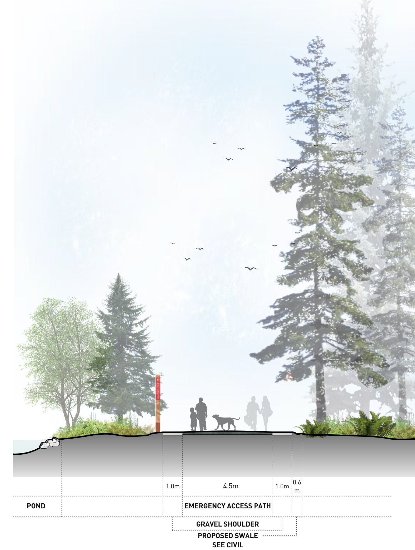
3 SECTION : THROUGH EMERGENCY ACCESS PATH Scale: 1:100
