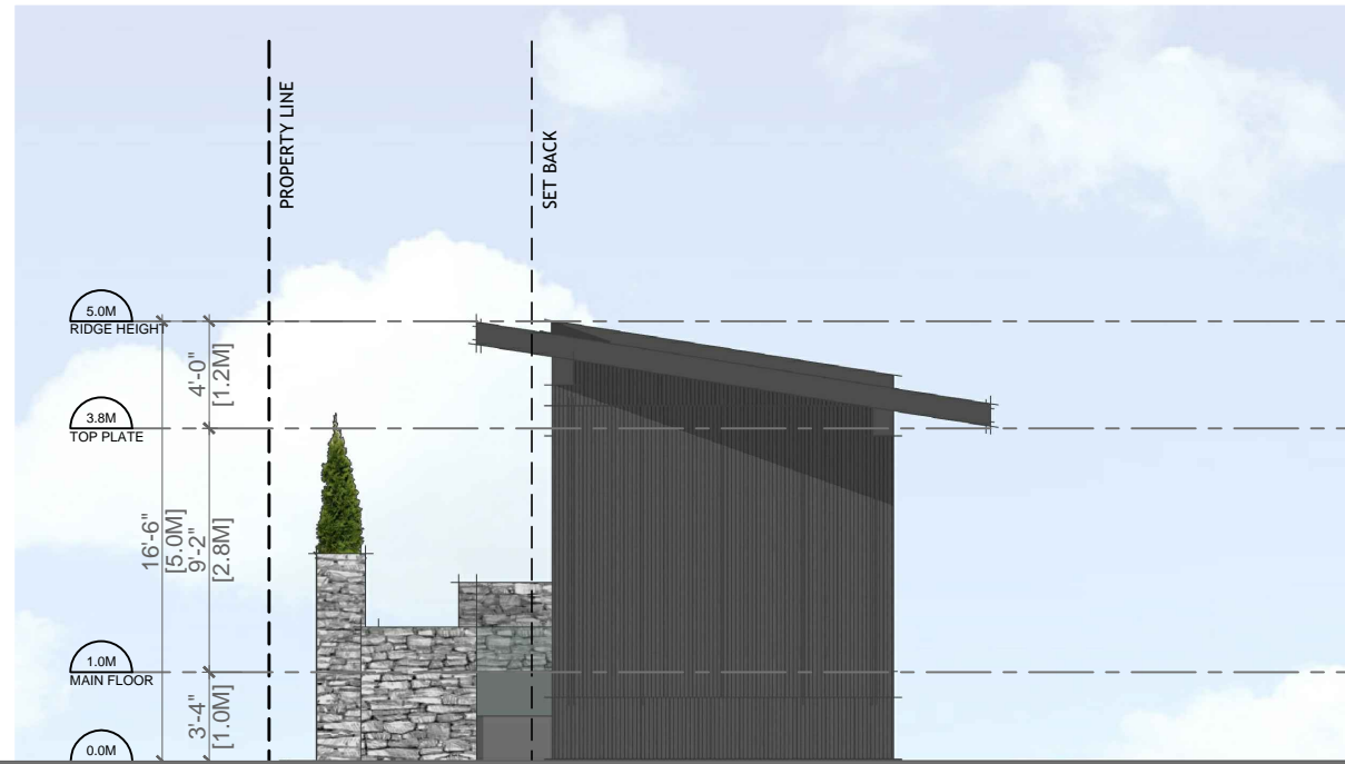
LEFT SIDE YARD ELEVATION 1/8"=1'-0"
