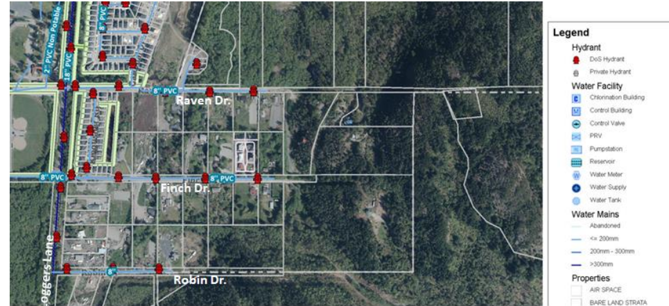
Figure 12 Existing Water Infrastructure
