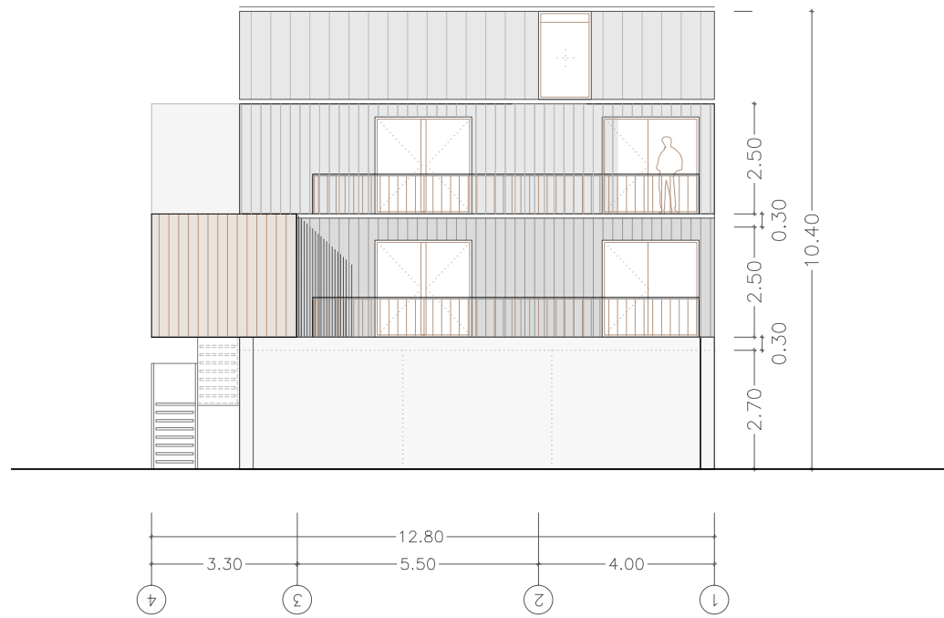
Front Lane Elevation__e 1/150
