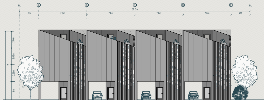
Sideyard elevation of a 4 unit rowhomes configuration showing entry courtyards, rooftop decks, and parking. 1:300
