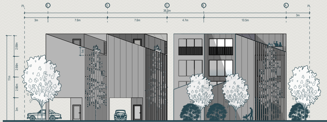
Sideyard elevation of a 4 unit cluster arrangement where 2 units are positioned at the front of the lot facing the street and two are at the rear facing the sideyard. 1:300
