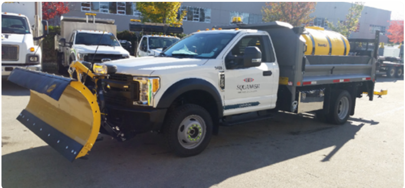
Figure 2.10.3) Image of a typical 4x4 truck with a mounted 9 ft (2.75 m) articulating nose plow, typically used for laneway or narrow road snow clearing.
