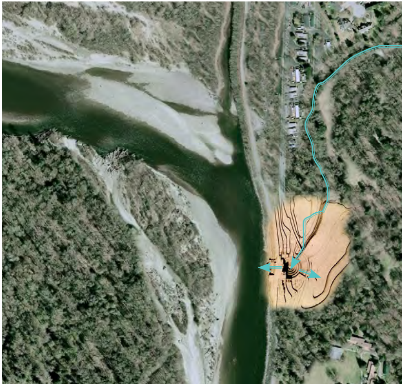
(Figure 6.21) A “switch” to direct the flow of water in the landscape. (Adapted from Google Earth imagery).
