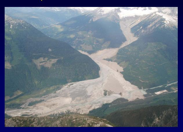
At km 8, the Mount Meager debris flow ran 270 m up the opposing wall of Meager Creek and then split, with one lobe of debris traveling up Meager Creek and the other down Meager Creek to Lillooet River
