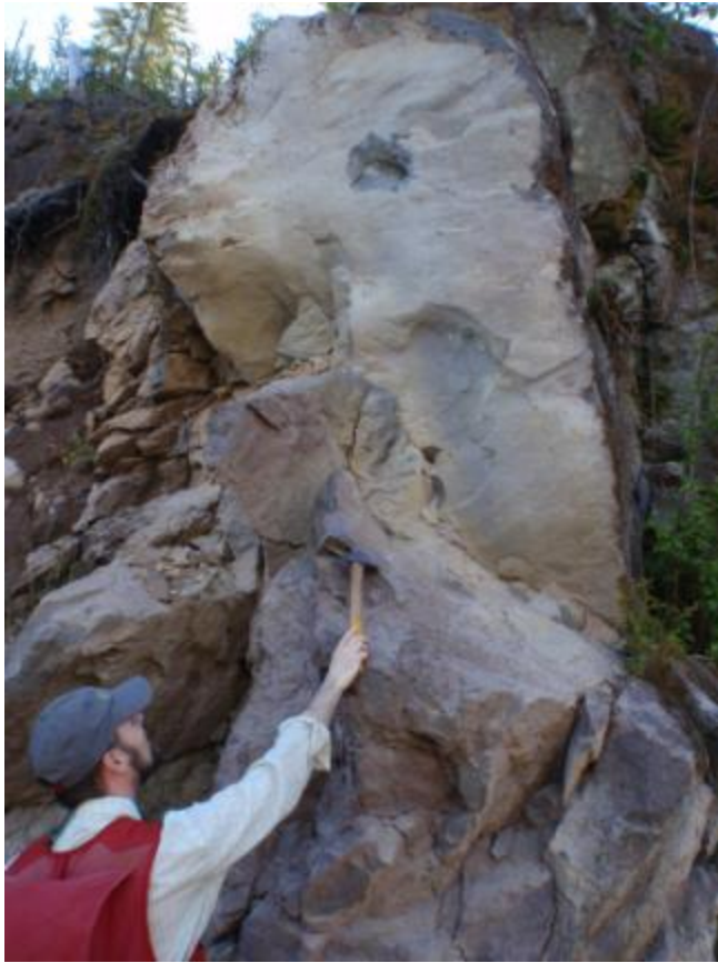
Photo 11. Weakly jointed and massive core of Ring Creek Lava Flow (June 15, 2012).
