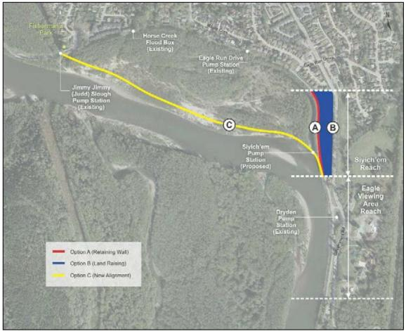
Figure 3-1: Conceptual Alignments of Shortlisted Options in the Siyich'em Reach
